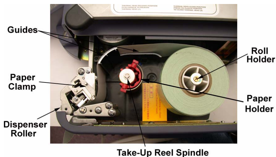
Figure 7-20. Loading DC-300 Printer
